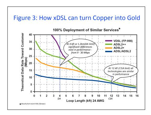
It may be observed from the characteristics that different DSL technologies can be differentiated at a loop length distance of 1.2 km. It may also be noted that beyond about 3 km, there is significant drop in throughput and consequently subscribers beyond 3 km upto the full range of 5 km that an exchange normally serves would not be enjoying the same throughput that is required for a good quality of experience.
